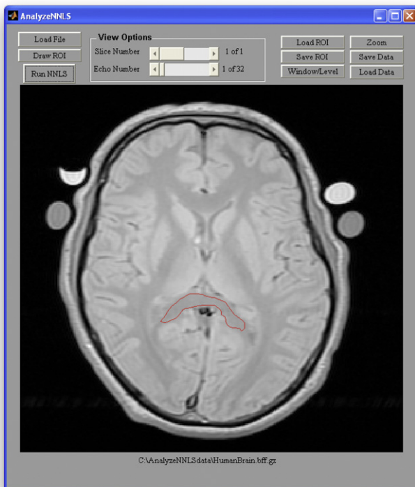
Fig. 2. Regions of interest are drawn using a function available in the Matlab image processing toolbox. Once the ROI is drawn an additional panel appears showing the decay of the signal averaged within the ROI for each echo (not shown). At this point more buttons are unveiled for further use.
